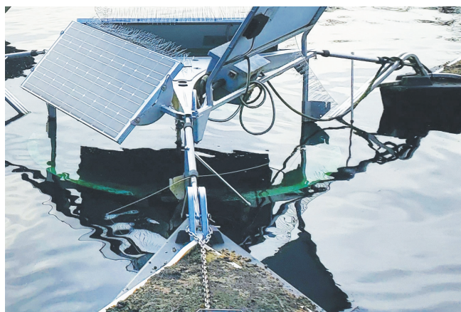
Surface Aerator with Solar Panel
