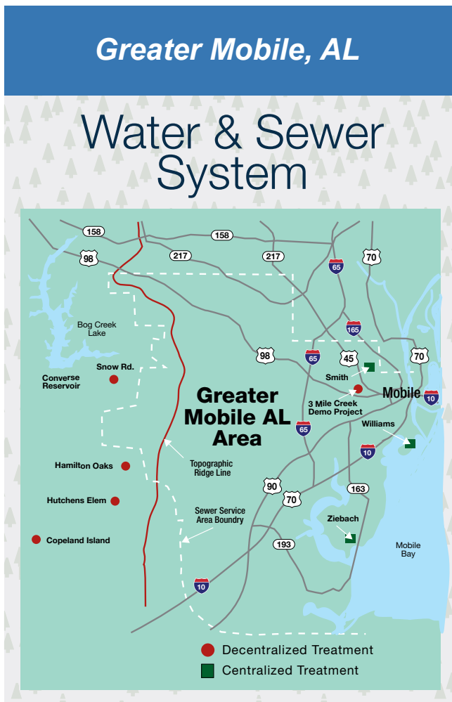
Existing WWTPs in green, proposed decentralized system as red dots, and ridgeline in red.
