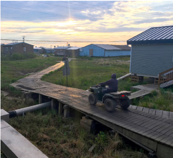
Evening sunset "downtown" Kotlik AK. (No roads in village, only boardwalks) Water and wastewater system is above ground, due to permafrost below ground.
